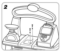
Remove the two existing screws from your counter top. Discard these screws.
